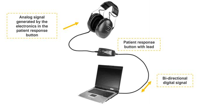
The DSP (Digital Signal Processor) located in the patient response button ensures communication with both the computer and the sound generation.
