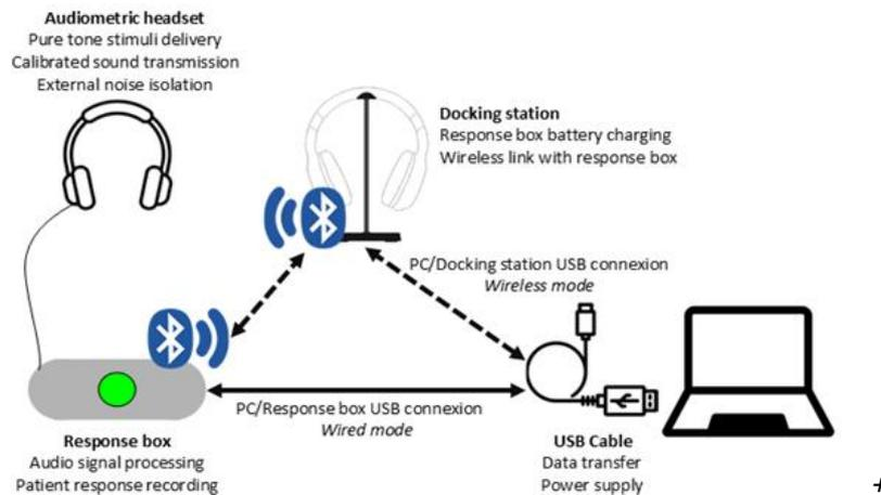
The Audiolyser® ADL Connect can be set up with different headsets depending on user needs (see section 6. Technical characteristics).
